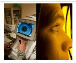
(L): Corneal Topographer with placido disc images on device screen.(R): Corneal Topographer with placido disc images reflecting off patient cornea. (Source L: U.S. Air Force photo by Airman 1st Class Kate Thornton/Released. Source R: U.S. Air Force photo by Staff Sgt. Perry Aston/Released)
